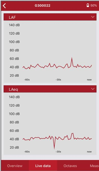
This screen displays live noise data for any two chosen parameters (which can be changed by pressing the arrows on the chosen parameter).
