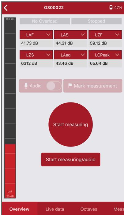
This screen is the default home screen for dBActive and displays live noise data for a number of parameters, each of which can be changed. Press the arrow on the value you wish to change. A menu will appear allowing you to select the value you wish to see (see image below).
