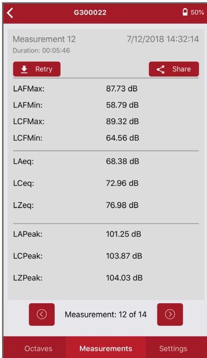
This screen displays the data for all main noise parameters. You can cycle through measurements by using the arrows at the bottom of the screen.
